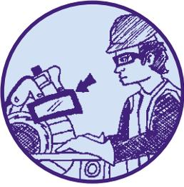
Many hand/portable tools have rotating shafts and components. Others emit fragments, dust and sparks. Such tools must have suitable guards fitted (eg, circular saw guards, power-take-off shaft guards, etc).
