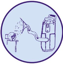
Tools and equipment which generate dust clouds should be fitted with extraction or wetting aids.
