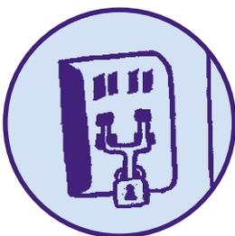
Where electrical power remains live, and subsequent work is required (including live work), isolation and tagging-off systems (including permit-to-work systems) should be used. All electrical work must be closely supervised by trained and competent electricians. The Electricity Regulations and the ETCI rules must be fully complied with.
