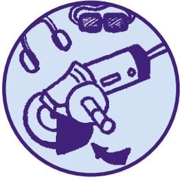
Angle Grinders must be maintained in good working order and regularly serviced. Guards must be in place at all times. Appropriate PPE (personal protective equipment) must be used.
