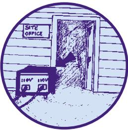
To avoid the silent killer, petrol and diesel-driven generators must always be used outdoors to avoid the deadly effects of the build-up of carbon monoxide from exhaust gases.
