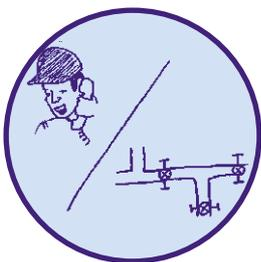
Before work near overhead or underground cables, gas services or other underground services begins, the relevant utility company must be asked to divert the service away from the work zone, or if necessary to switch off or stop the service temporarily to allow work to proceed safely. Contact with overhead lines can kill. Never erect scaffolding or similar structures close to or under live overhead lines. Never work close to, or access close to, or under live overhead lines.
