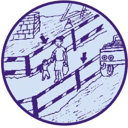
Where members of the public have to access close to, or around construction work, suitable safe routes must be provided to protect them. Consideration must be given to people with disabilities. Construction debris must be kept clear from such public areas. Muck, dust, trip hazards, protruding puncture objects and objects likely to fall, etc, must be removed. Where reinstatement is required, it must be completed without delay.
