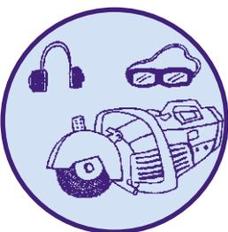
Consaws, which are widely used on construction sites, must be maintained in good working order and regularly serviced. Guards must be in place at all times. Appropriate PPE (personal protective equipment) must be used.
