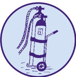
Gas bottles must always be stored upright, and chained to prevent falling. Flash-back arresters must be used on gas bottles. All flexible hosing and connections should be checked daily, and any damaged parts replaced prior to use.
