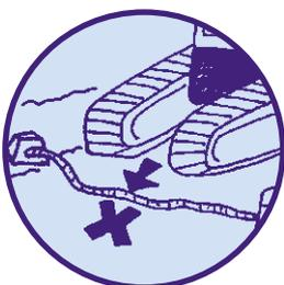
Trailing electric cables which would risk being damaged because of their position must be protected from such damage, or else they should be placed in a safe location.
