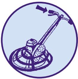
Power floating is the process of levelling concrete floors. Power-floating equipment should be regularly serviced to ensure it is in good working order. Damaged or worn handgrips should be replaced immediately. All guards must be kept in place. If power-floating takes place close to open edges, adequate edge protection must be provided.
