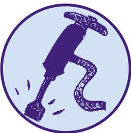
To reduce and eliminate the risk of ill health due to vibration, jack hammers and kangos must be serviced regularly and maintained in good condition. Jack hammers should not be used for long periods. Workers may be rotated to other tasks to reduce exposure time and prevent vibration-
