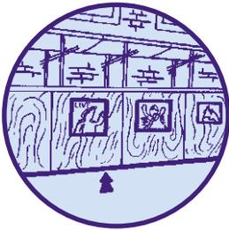
Particularly on street-side works, adequately designed and constructed hoarding should be erected to secure construction work. Arrangements must be put in place to ensure that normal pedestrian and public vehicular traffic is not put at undue risk, as a result of any changes made.
