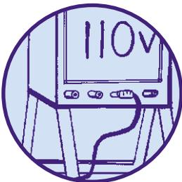
All portable electric tools rated below two kilowatts that are used on construction sites must be rated at 110V.
