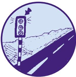
Traffic-control plans must be prepared, to help control traffic movement especially at the entrance and exit of any construction site. These may include warning signs, bollards, stop-go systems, ramps, temporary traffic lights, stop-go men and flagmen. Liaison with local gardaí may also be necessary. The Department of the Environment's Traffic Signs Manual should be referred to.
