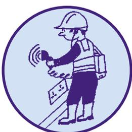
Before drilling or cutting begins, the area should be scanned with a detector to verify the position of any services. The position of the service should be carefully marked, to ensure that subsequent work does not come into contact with it.
