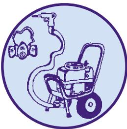
Spray-painting equipment must be set up in accordance with the manufacturer's guidelines. It should undergo regular service and maintenance checks. To prevent others coming into contact with spray products, exclusion zones need to be set up.
