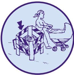
All ongoing works – in particular street-related activities, open excavations, exposed manholes, etc – must be protected with barriers and identified with warning signs.
