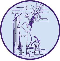
Welders and flame cutters must only be used by competent, qualified persons. Suitable PPE (personal protective equipment) must be provided and used. A fire extinguisher and sand bucket along with appropriate screens must be readily available during cutting and welding. In many situations where hot working is used, a permit-to-work system should apply to prevent the risk of fire and explosion.
