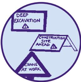
People approaching construction work must be given advance warning, especially where specific hazards exist. Warning signs must be erected and, where necessary, must give clear directions to passing members of the public.
