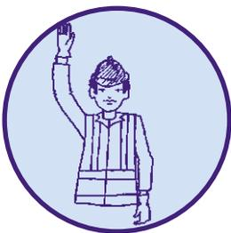
A banksman (a trained slinger and signaller) must always be used where loads are lifted, and safe direction is given to operators of lifting appliances.
