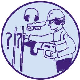
Use of cartridge tool guns and staplers requires careful planning, to assess what will be fired into, and who or what may be behind the target. People should be kept a safe distance from the firing zone. Whoever uses these tools should always wear goggles and ear protection. Such tools must be maintained in good working order, and should be operated only by trained persons.
