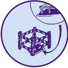
Where services have been uncovered or made visible, and remain visible or are insufficiently backfilled, suitable barriers should be erected at a sufficient distance around the service area to protect and warn drivers of plant and others of the danger.
